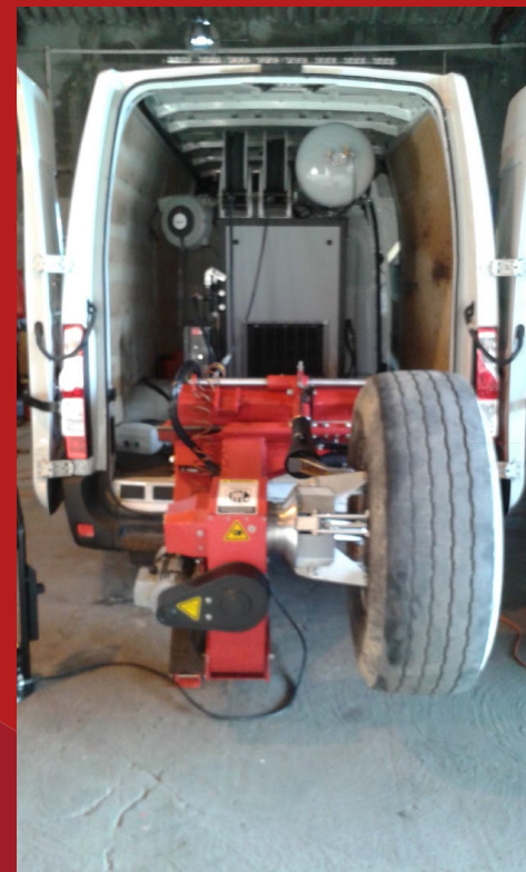
INSTALLATION AT REAR DOOR WITH INVERTED CHUCK
